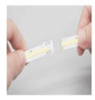
Insert each ends of led strips into the end of the connection terminal respectively, make sure the metal clip is on the same side as the metal solder pad of led strip.
